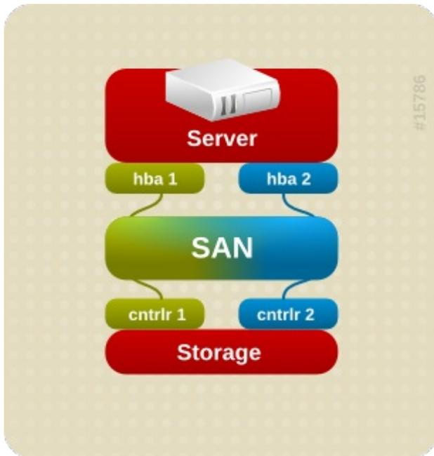
Figure 1.3. Active/Active Multipath Configuration with One RAID Device
